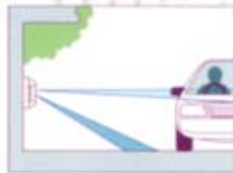
When only the upper zone detects a moving object, the unit is not activated.
