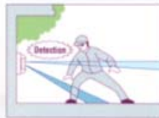
When both the upper & lower zones detect a moving object, the unit is activated.
